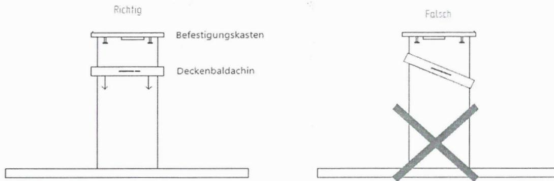
**ATTENTION: Always keep the ceiling canopy horizontal when moving it and always keep the guide cables slightly taut, so that they are not damaged.**
