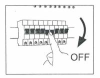
Always turn off the power before installing the lamp.
