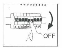
Always turn off the power before assembling the lamp.
