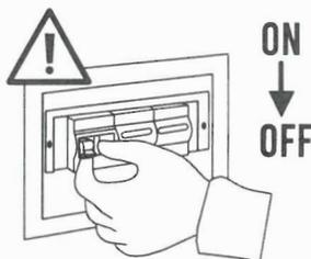
EN- Turn off the mains before installing the lamp.
