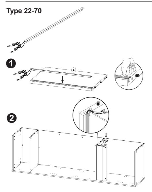
Verkabelung => Montageanleitung 22-70-K / 22-89-K cabling = assembly instruction 22-70-K / 22-89-K
