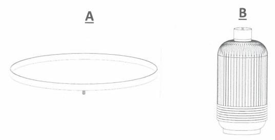
• To assemble the product, please turn the enclosed part A on the part B in the clockwise direction .
